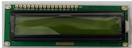
Figure 2: 16x2 LCD display
