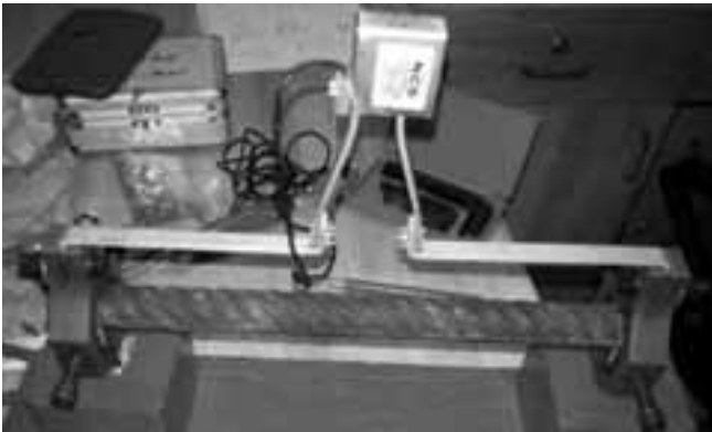
Fig. 4: Holding fixture and increment accessories on existing extensometer
