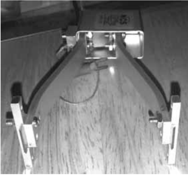
Fig. 3: An Existing Extensometer with 50mm gauge length
