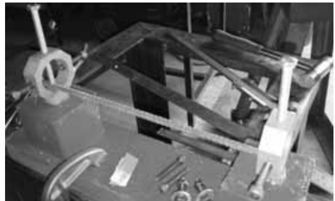
Fig. 5: Fabricated fixture holding 8mm diameter TMT bar with predefined 300mm gauge length
