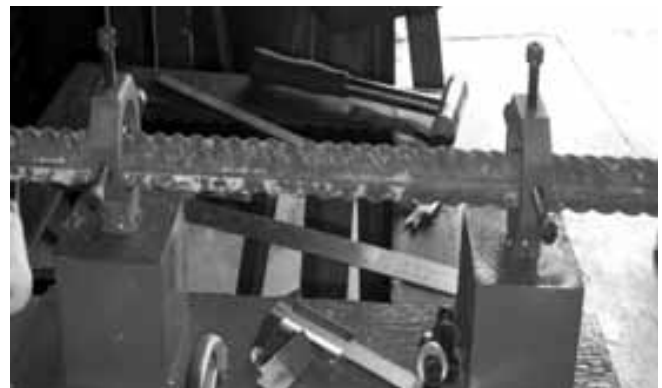
Fig. 6: Fabricated fixture holding 30mm diameter TMT bar with predefined 300mm gauge length
