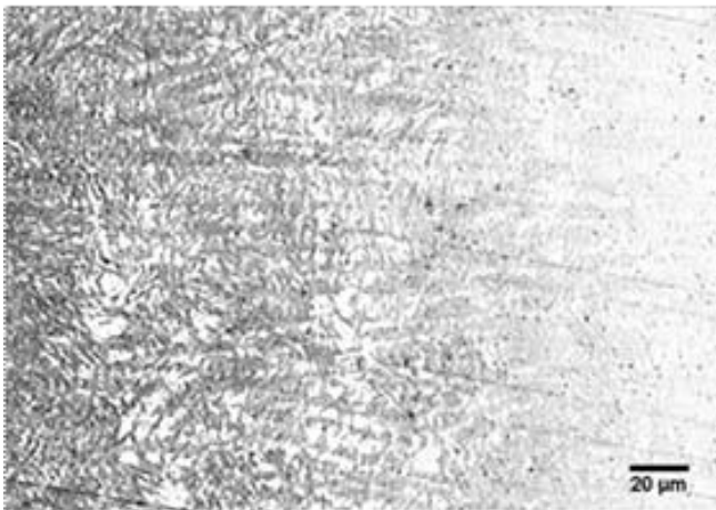
Fig. 6: Ni-Fe alloy, weld metal in first layer
