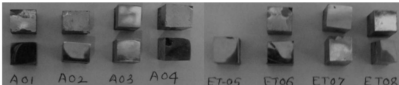
Fig. 1: Specimen showing buttering layers
