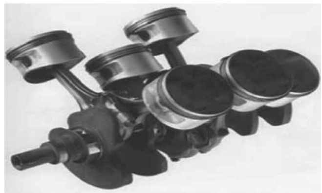
Fig. 1: Typical Diesel Engine Pistons
